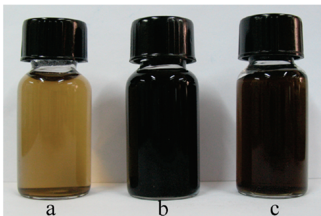
Figure 9. Photographs of aqueous dispersions (0.1 mg/mL) of GO before (a) and after the reduction with fructose (b) and sucrose (c) under the same reaction condition as with glucose.
